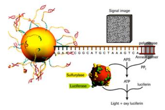
Figure 1. Sequencing-by-synthesis with the GS FLX (454 Life Sciences): During the incorporation of a nucleotide though polymerase activity, PPi is released and converted into ATP. Upon contact with the enzyme luciferase, light is released, which is recorded by a camera. (source: 454 Life Sciences: <u>http://www.454.com/products-solutions/how-it-works/sequencing-chemistry.asp</u>)
